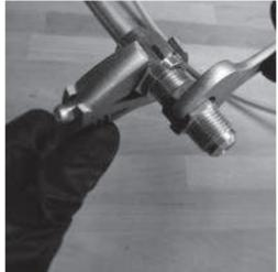
6. Inspect the joint: unscrew the IGLOO QUICK fitting and repeat the steps from 3 to 5: at step 5 tighten the joint with a common wrench for not more than 1/4 of turn (90°). Note: Don't use a dinamometric wrench.
