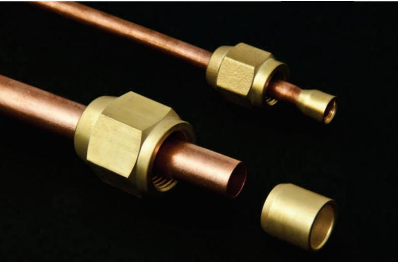
IGLOO QUICK nuts allow the union of tubes in a few seconds: just push-in the tube and screw 1 and ½ turn with a common wrench. Flaring tool and dinomometric wrench are not required.
