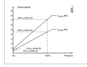
The diagram indicates the relationship between output signal from AKS 32R, supply voltage and pressure.
