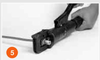
5 Crimp the ferrule with our RXA005 hydraulic pliers until the pliers automatically click. The pliers will open automatically.
