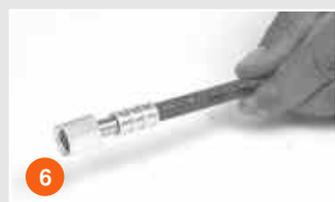
6 The assembling process is finished. Check to make sure that the components are positioned correctly and the crimping.
