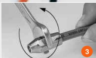
3 By hand, screw the ferrule counterclockwise onto the capillary hose. When it becomes too hard, finish screwing with a wrench until it can't go any further.
