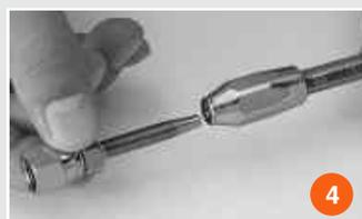
4 Connect the insert piece to the ferrule. By hand, screw the insert piece counterclockwise onto the capillary hose.
