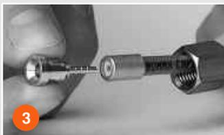
3 Make sure that the ferrule is positioned on the very end of the capillary hose, ready to connect to the next piece. Connect the insert piece to the ferrule.
