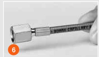
6 The assembling process is finished. The nut can slide freely over the ferrule: check the correct positioning of the components and the crimping.
