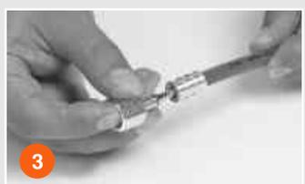
3 Connect the insert piece and the nut simultaneously onto the capillary hose.
