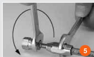
5 When screwing by hand becomes too hard complete screwing with a wrench and skeleton key.
