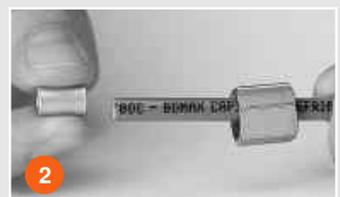
2 Insert the nut onto the hose keeping the threaded end turned towards. Insert the ferrule onto the capillary hose.
