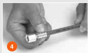
4 Make sure to insert the insert piece entirely and tightly fitted into the ferrule. Next, carefully slide the ferrule towards the remaining part of the insert piece.
