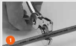
1 Cut the Quadra DN4 capillary hose to the required length using the special WXA004 cutter.
