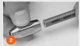
2 Insert the ferrule onto the capillary hose.
