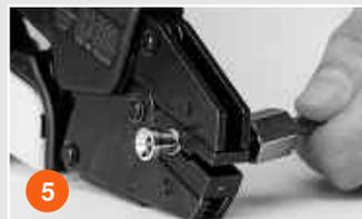
5 Crimp the ferrule with our RXA003 hand pliers until the ferrule automatically click. The pliers will open automatically.
