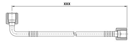
Straight female 1/4 (with valve opener) + elbow female 1/4
